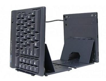
Ascent is 2 sturdy steel tenting modules which attach to the underside of the keying modules. A linking plate connects them and allows tenting from 20 to 90 degrees in 10 degree increments. Can be used with 230mm lead but is best with 510mm lead. Palm supports optional at 20, 30 and 40 degrees.
